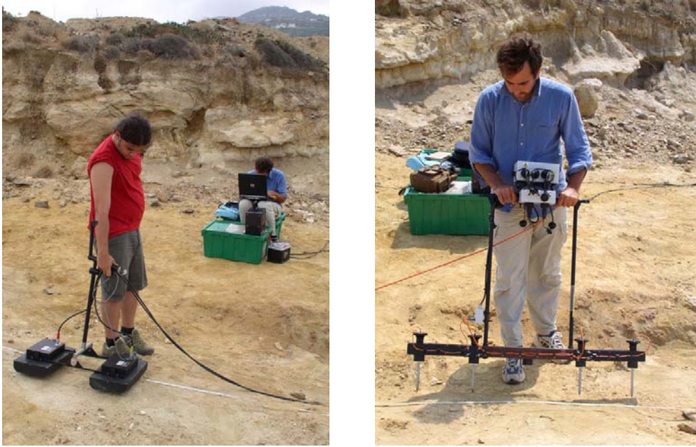
Figure 2. The EKKO1000 ground penetrating radar (left) and the Geoscan Research RM15 resistivity meter were employed in the geophysical investigations of the site of Gela.
