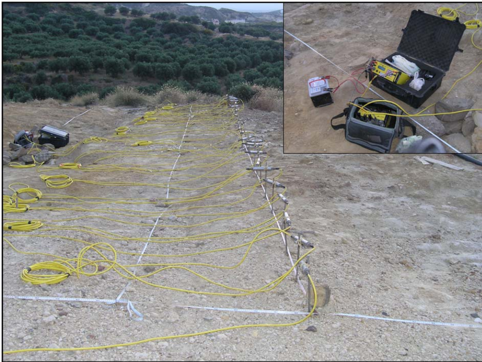
Figure 3. The Sting Advanced Resistivity Tomography package and the layout of the electrodes for measuring the electrical resistance of the soil through the dipole-dipole configuration.
