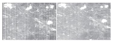
Fig. 1. Hyperion band 8 (436nm) uncorrected image (left), and corrected using Spectral Moment Matching and local destriping (right).
