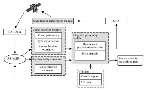
Fig. 7. The architecture of the Remote Sensing Monitoring System for Maritime Search and Rescue (RS-MSR)
