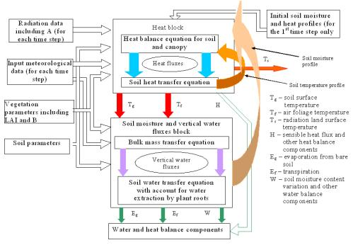
Fig. 6. The SVAT model flowchart
