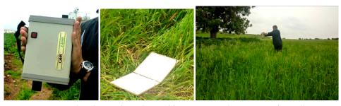
Fig. 6. GER 1500 used in this study with its calibration target (Agapiou et al. 2010)
