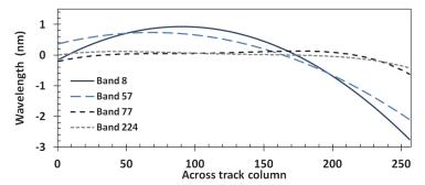
Fig. 2. Laboratory measured spectral shift of Hyperion (Barry, 2001).
