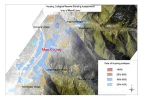
Fig. 5. The damage assessment result of Maoxian County for houses.
