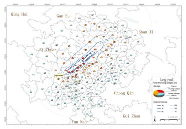
Fig. 8. Comprehensive assessment map of damage for houses
