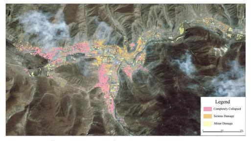
Fig. 21. Housing damage assessment results
