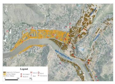
Fig. 29. Housing damage assessment map
