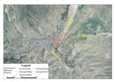
Fig. 30. Road and bridge damage assessment map
