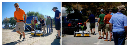
Sensys array of fluxgate gradiometers, Sensys being pulled by car, MALA MIRA 8-channel GPR system being pulled manually and with vehicle.
